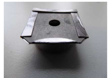
Fig. 3: Liner with perforated cover
