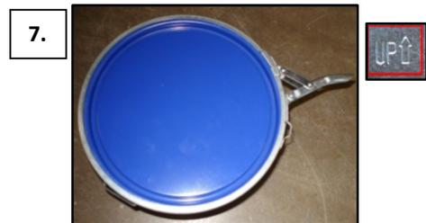
**Step 7:** Don a pair of cut resistant gloves. Place Leverlock ring over pail lid – Confirm "UP" indicator is in correct orientation on ring. Place over pail and while using downward pressure on pail lid secure Leverlock Ring. Apply tamper evident zip-tie to Leverlock. Affix fully completed Customer Return Container Condition Form on the outside of the pail or box (Step 8).
