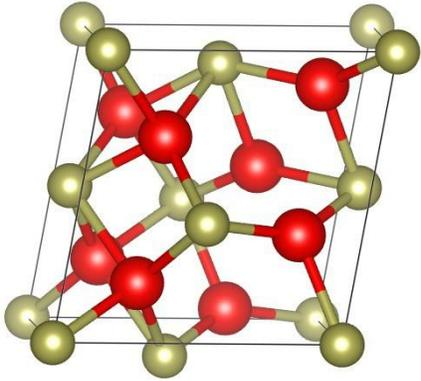
A **monoclinic phase** ( $P2_1/c$ ) is the *most stable phase* at room temperature and standard pressure, but is **not ferroelectric**.
