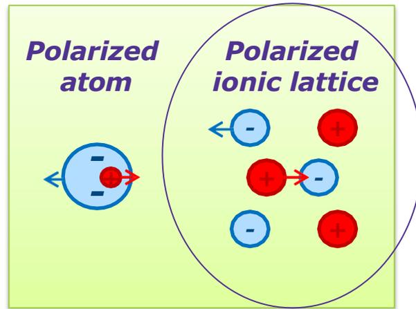
Ferroelectrics have an apparent "stored charge" called the "remanent polarization,"  $P_r$
