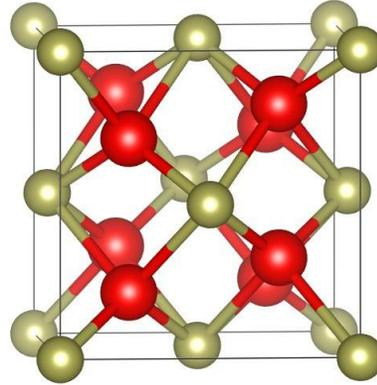
A **tetragonal phase** ( $P4_2/nmc$ ) has a very high theoretical dielectric constant ( $\kappa=75$ ) and a large bandgap ( $E_g = 6$  eV). It can also produce **anti-ferroelectric-like behavior**.
