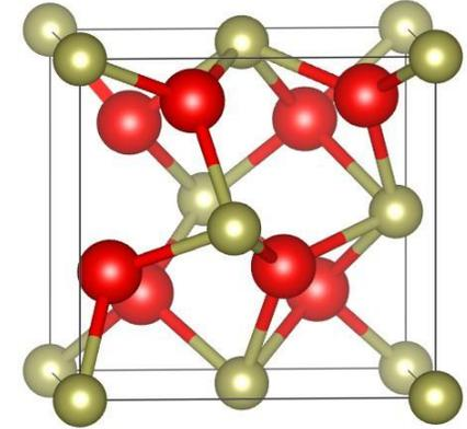
An **orthorhombic phase** ( $Pca2_1$ ), a metastable structure, is not centrosymmetric, and can therefore demonstrate **ferroelectric behavior**
