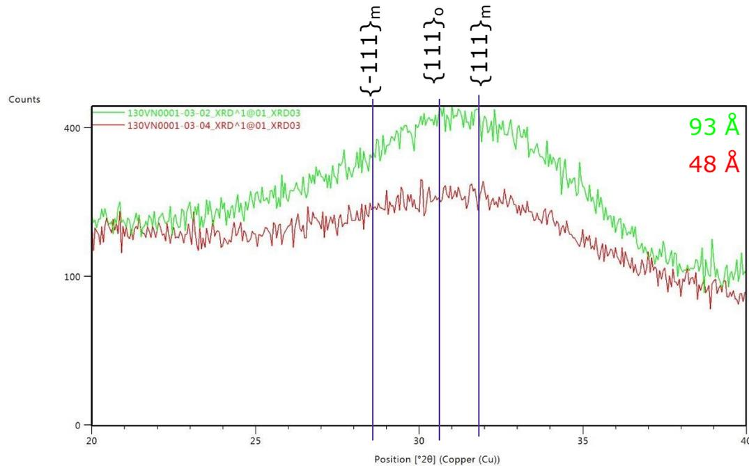
Ozone,  $T_{\text{dep}} = 300^\circ\text{C}$ , After 500°C anneal
