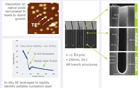
Utilizing Intermolecular's materials innovation platform, a suitable nucleation layer was identified and deployed to release continuous, conformal coatings of elemental Te on high aspect ratio test structures.
