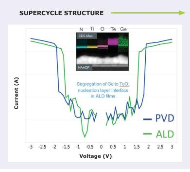
3X [Ge(OEth)<sub>4</sub>+((CH<sub>3</sub>)<sub>3</sub>Si)<sub>2</sub>Te  $\rightarrow$  GeTe<sub>2</sub>] (ref 1) 1x [((CH<sub>3</sub>)<sub>3</sub>Si)<sub>2</sub>Te+Te(OEth)<sub>4</sub>  $\rightarrow$  Te]
