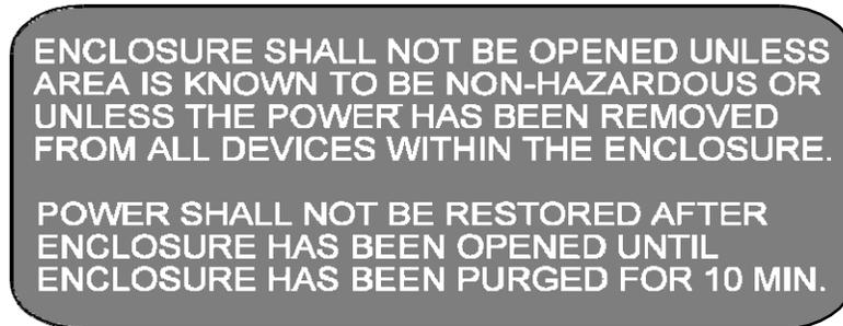
The following label appears inside cabinets containing cylinders. It is located on the inside door, approximately at eye level. It is also located on the cylinder strap on both cabinets and racks.
