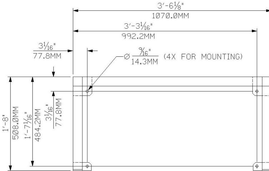
**Figure 2.2.2.4: Mounting Hole Locations**
