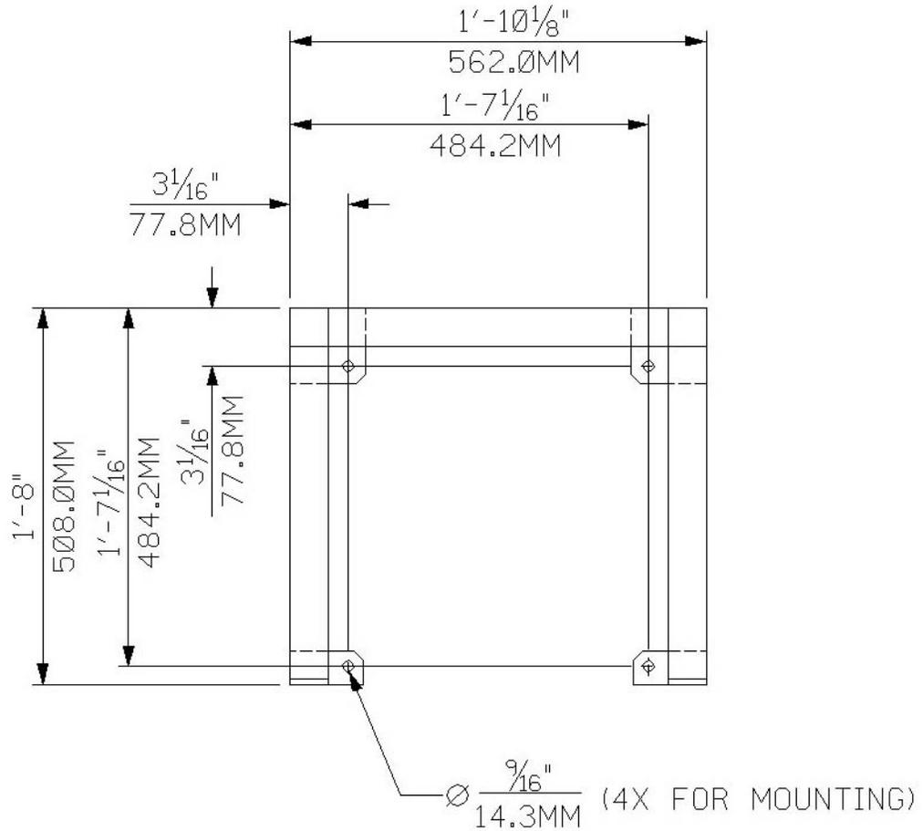
**Figure 2.2.2.1: Mounting Hole Locations**
