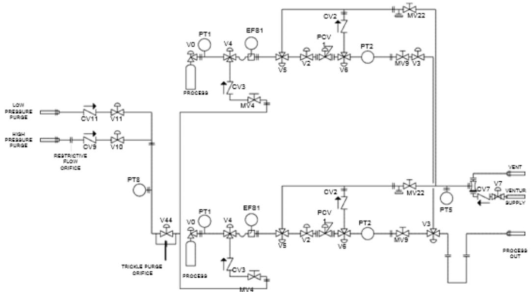
**Figure 7.12:** Example HPLT Piping Schematic
