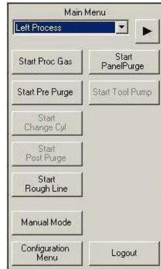
15. When the controller status box indicates "PRE PURGE COMPLETE", press the "START CYL CHANGE" pushbutton.
