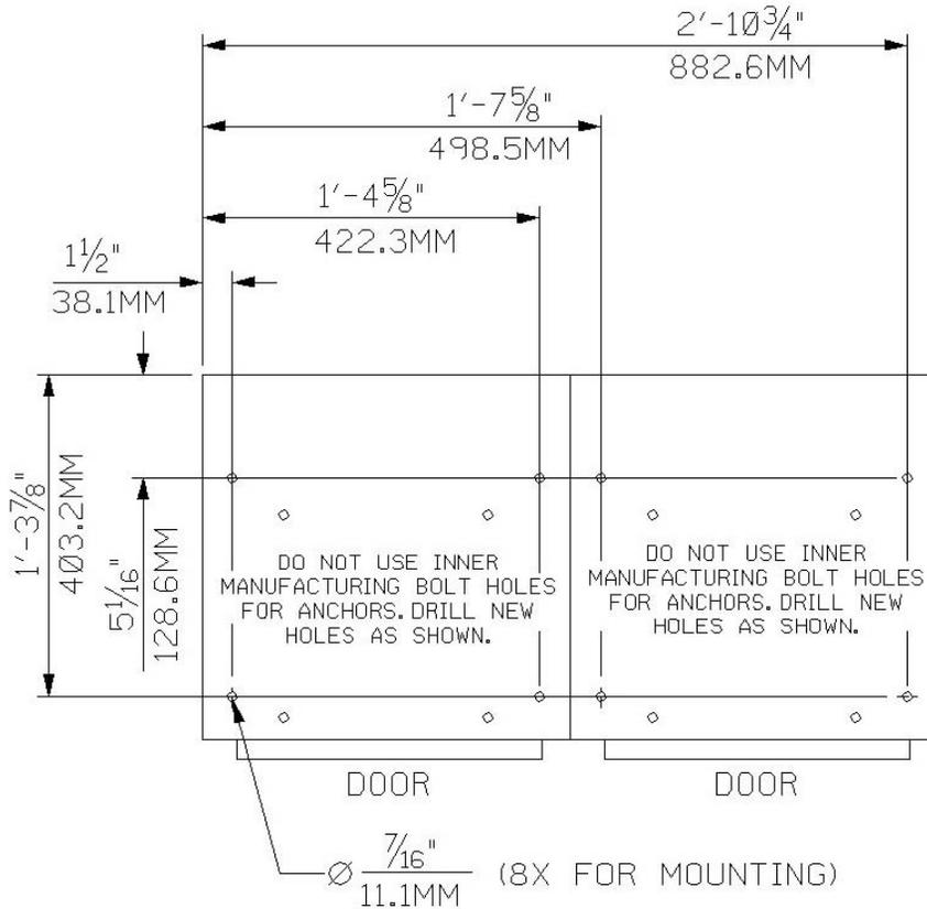
**Figure 2.2.1.4: Mounting Hole Locations**
