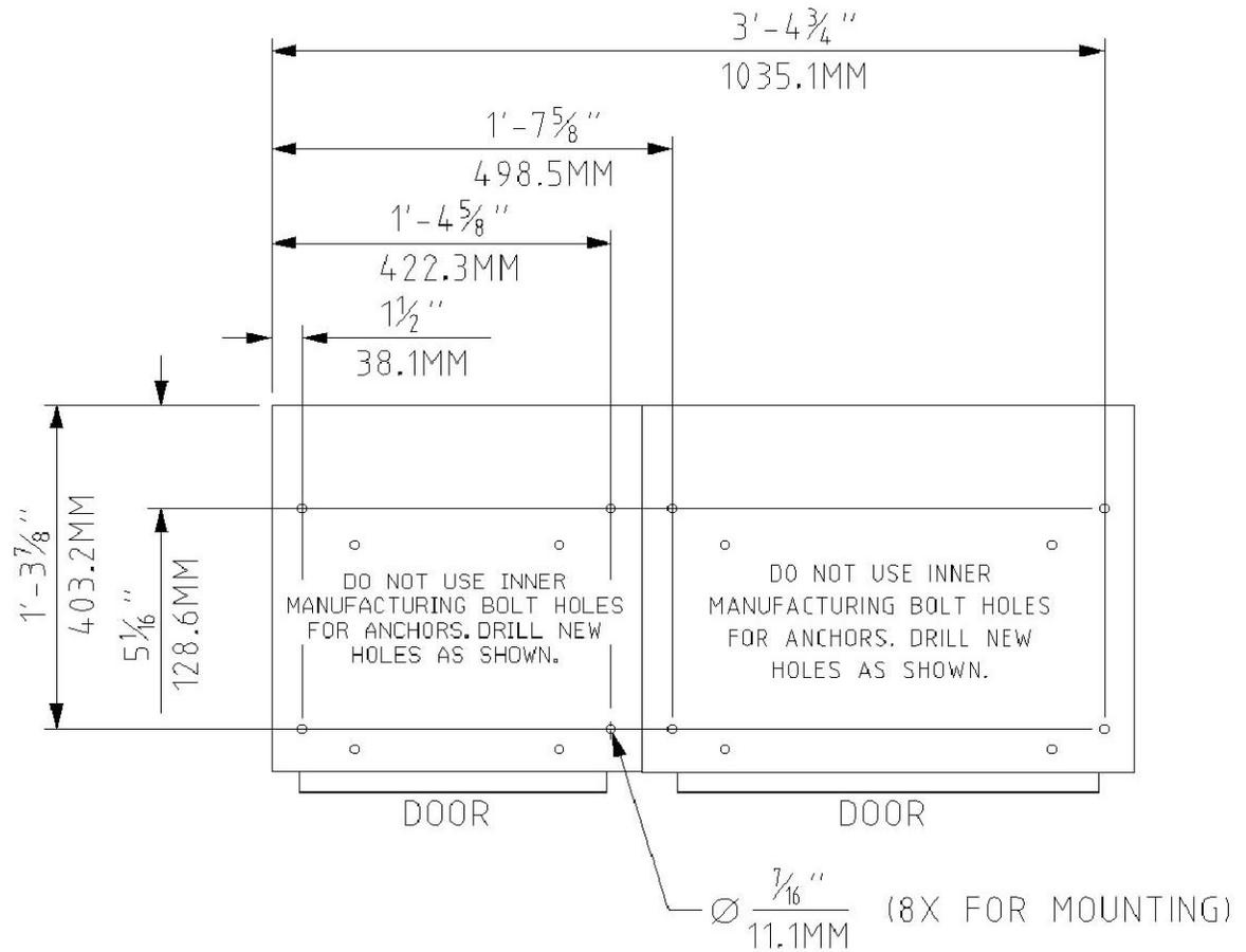
**Figure 2.2.1.5: Mounting Hole Locations**
