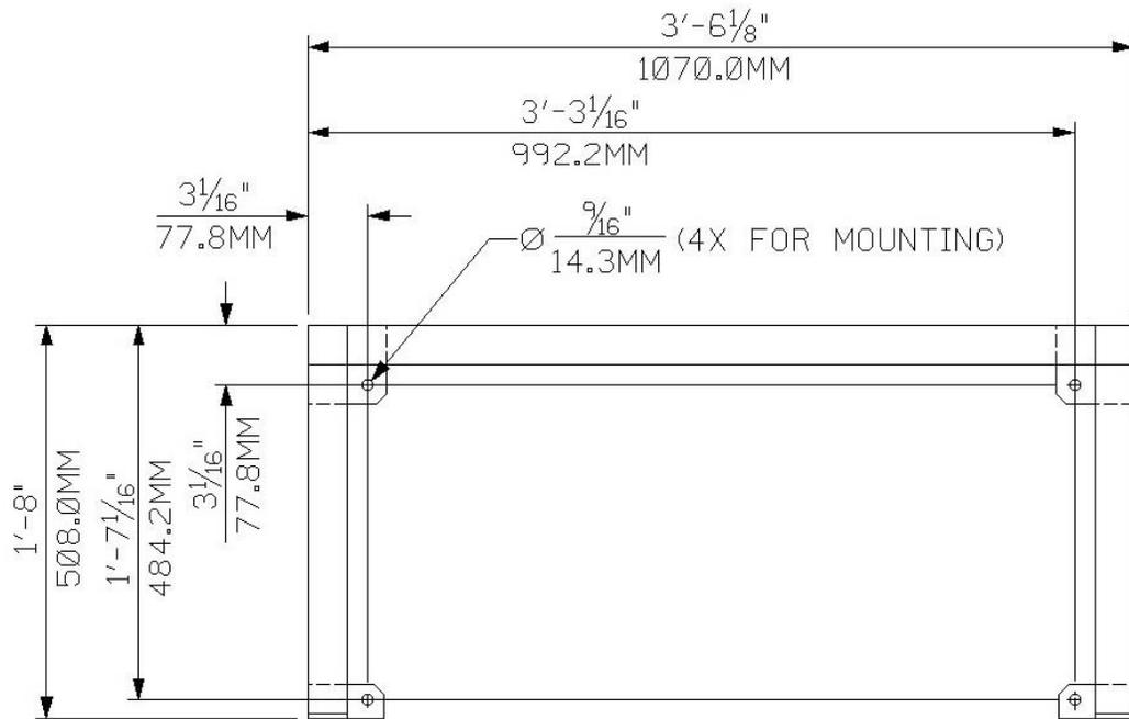
**Figure 2.2.2.3: Mounting Hole Locations
