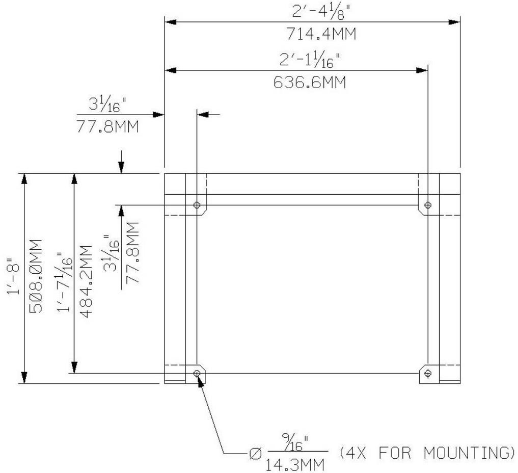
**Figure 2.2.2.2: Mounting Hole Locations**
