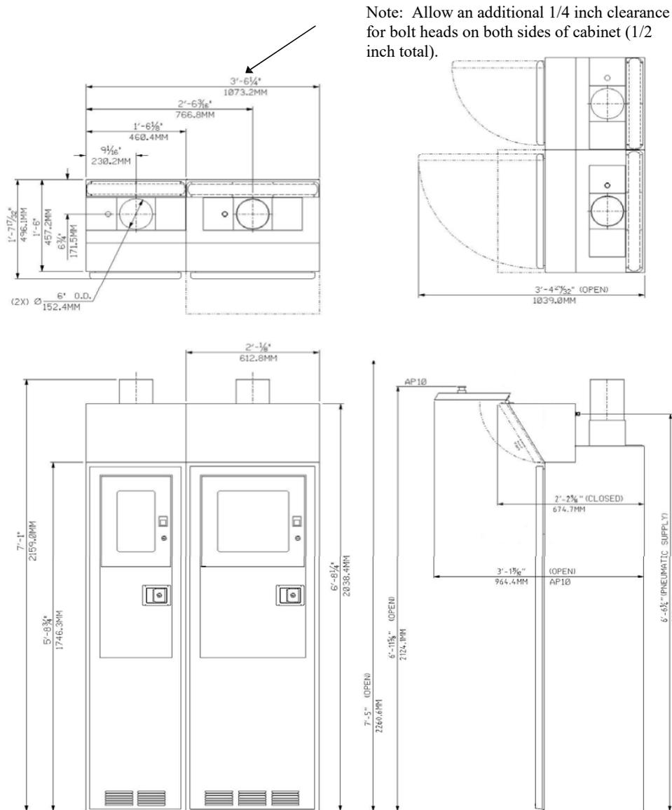
Note: Allow an additional 1/4 inch clearance for bolt heads on both sides of cabinet (1/2 inch total).
