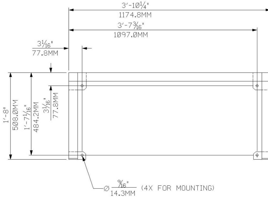
**Figure 2.2.2.5: Mounting Hole Locations**
