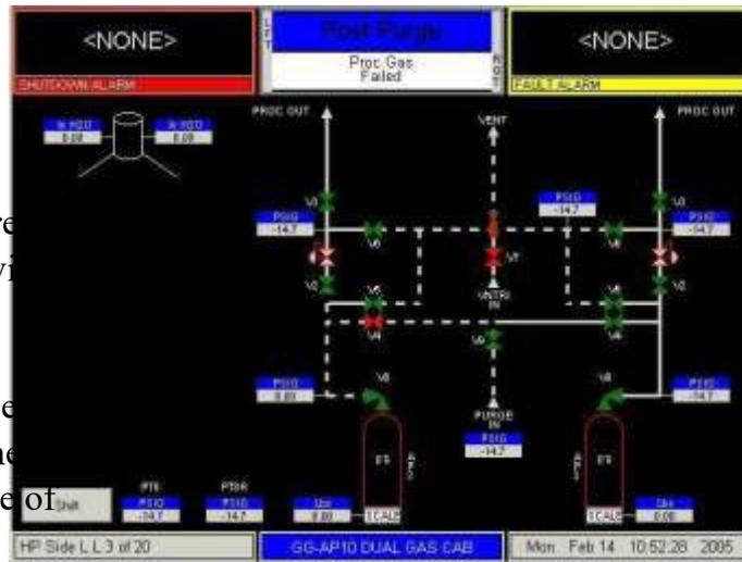
This sequence of evacuation and pressurization will be repeated until the configured number of cycles is completed.
