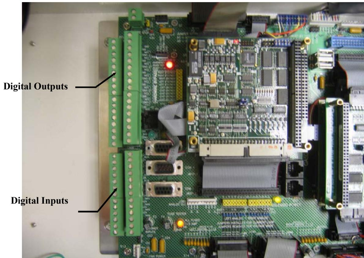
**Figure 4.6:** I/O Terminal Blocks
