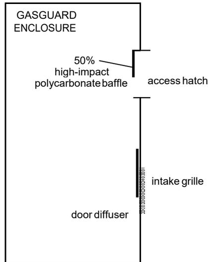
**Figure 3.6:** Exhaust Hook-up and Ventilation Measurement Location
