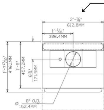
Note: Allow an additional 1/4 inch clearance for bolt heads on both sides of cabinet (1/2 inch total).
