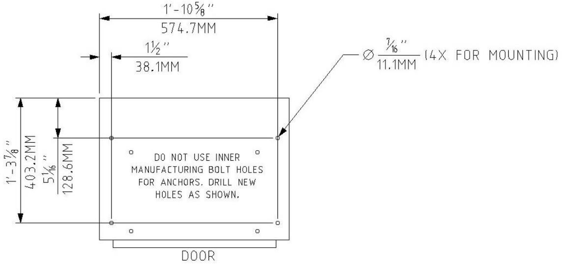
**Figure 2.2.1.2: Mounting Hole Locations**
