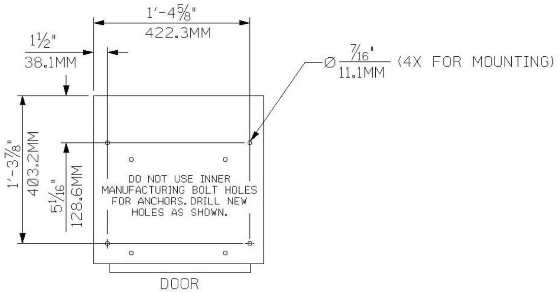
**Figure 2.2.1.1: Mounting Hole Locations**
