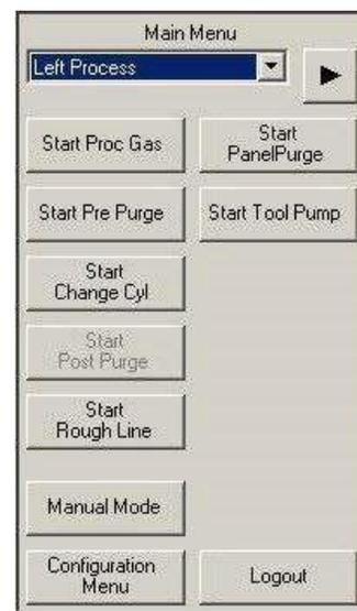
18. When the controller status box indicates "CYL CHANGE COMPLETE," press the "START POST PURGE" pushbutton.
