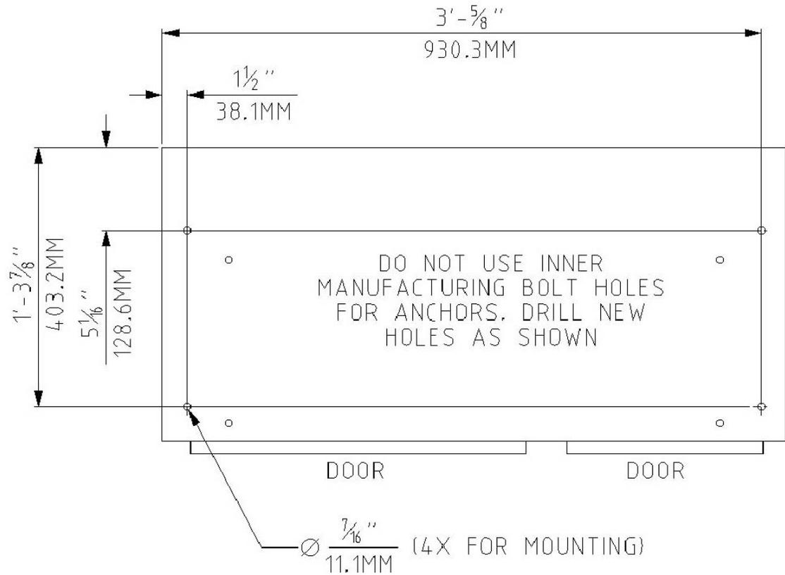
**Figure 2.2.1.3: Mounting Hole Locations**
