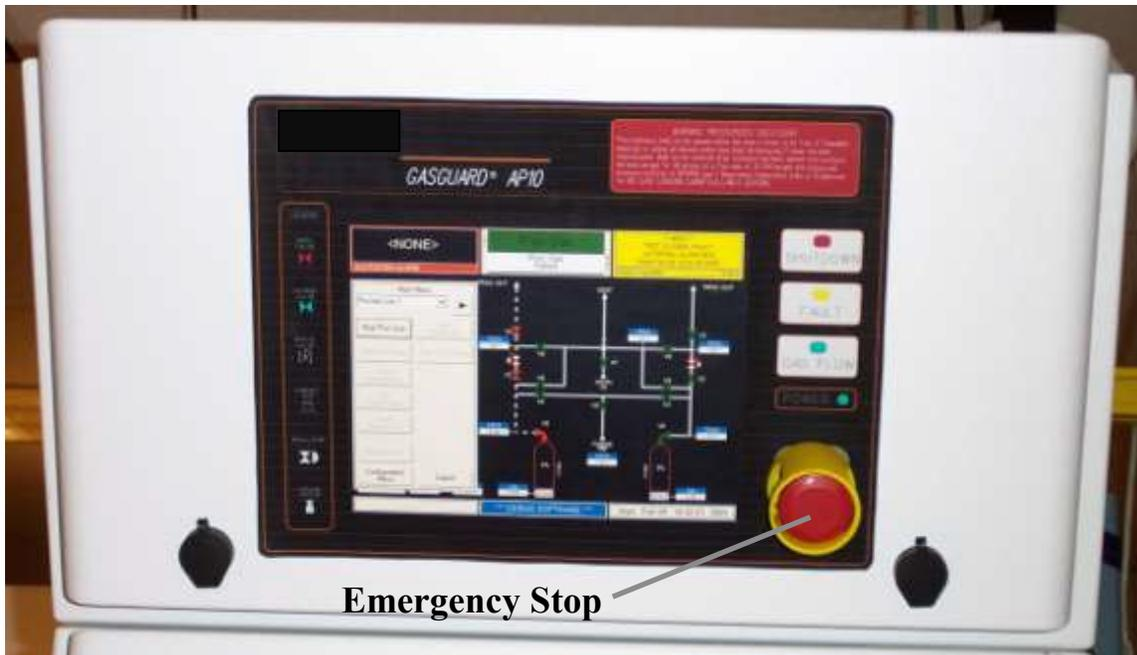
**Figure 8.1: Emergency Stop Pushbutton Location**
