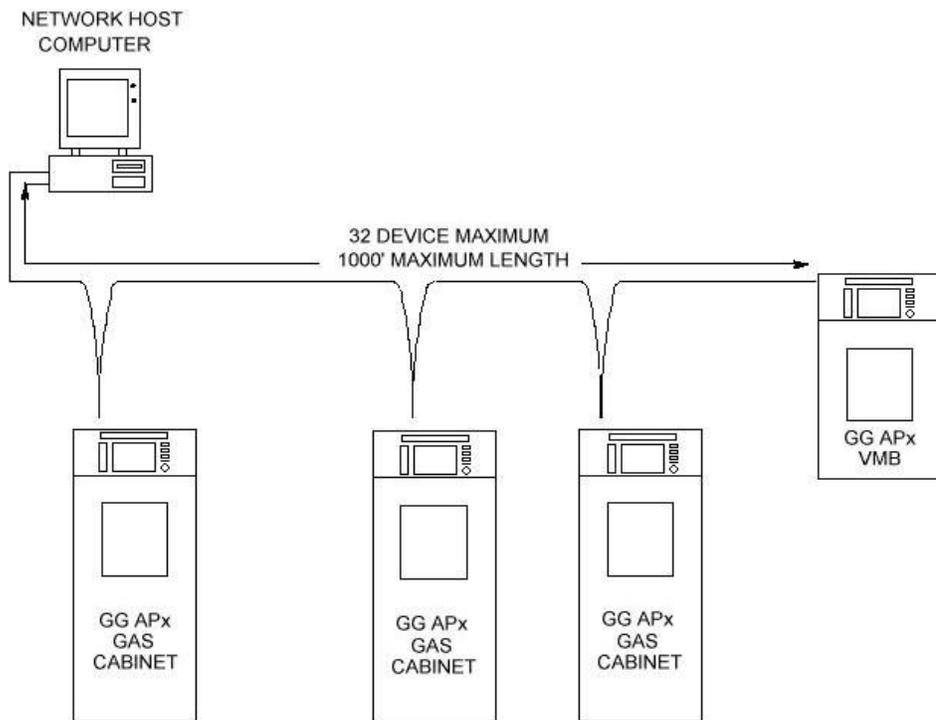
**Figure 4.13:** Daisy-Chain RS-485 Network Wiring Configuration
