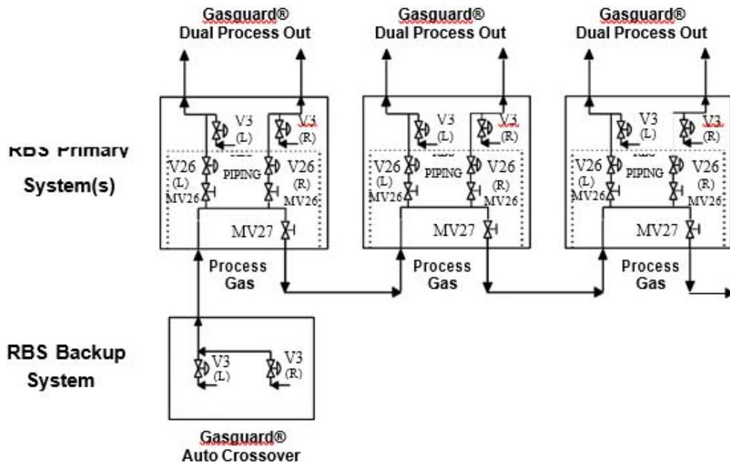
**Figure 7.9:** RBS - Simplified Piping Interconnections
