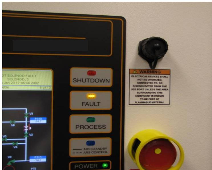
Figure 2-11: AP11 Controller USB Port on the Face of the Controller
