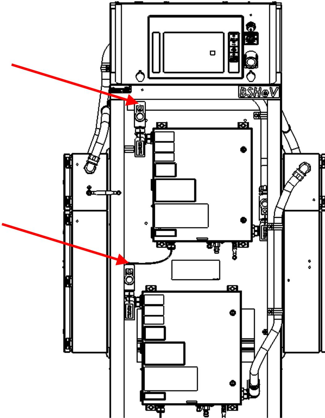
Figure 2-4: Heater Power Conduit connections
