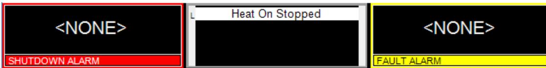
**Figure 3-5: Alarm and Controller Status Boxes**
