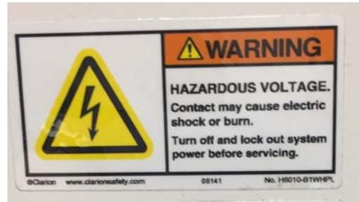
The following label is located on the front of the GASGUARD® AP11 controller adjacent to the USB port. Do not connect to the USB port unless the area is known free of flammable material.
