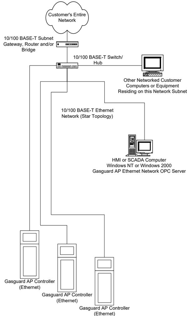
**Figure 2-15** Typical GCS Network Architecture
