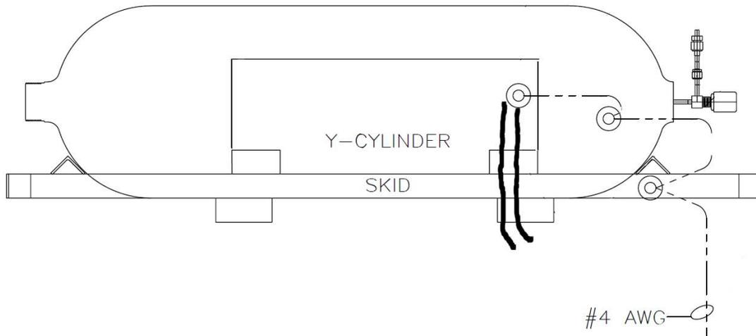
**Figure 4-13a: Cylinder/Heater Grounding**
