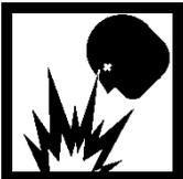
*In classified hazardous areas – Do not separate electrical terminations or connectors while energized due to risk of electrical arc or spark which can ignite potentially flammable atmospheres.*
