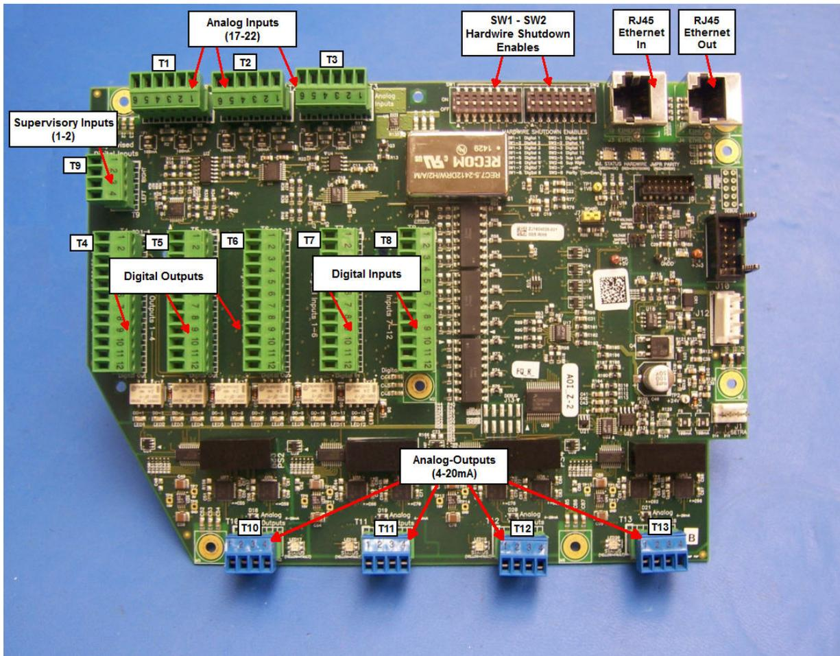
**Figure 2-5:** AP1580 Customer I/O Terminal Blocks
