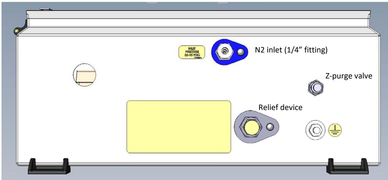
Figure 4-15: Underside View of BSH eV ECC
