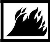
***This symbol represents flammable gases. Gases used with the GASGUARD® can cause flammable atmospheres.***
