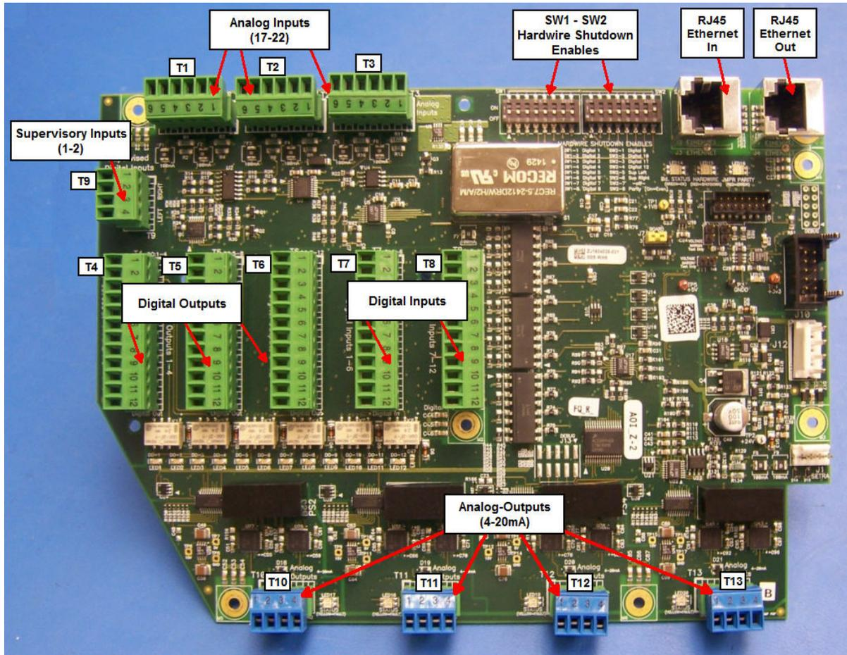
**Figure 3-8:** AP1580 Expansion Customer I/O Terminal Blocks (AP1563 board shown)
