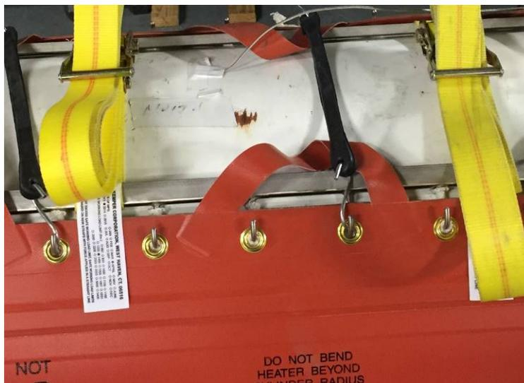
**Figure 4-11: Hooks attachment on the Grommet.**
