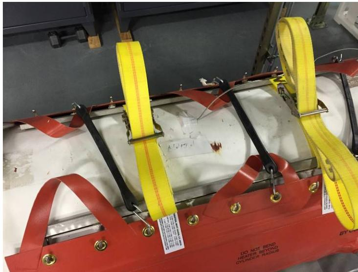
**Figure 4-9: Installation of stainless steel bars, rubber straps, and ratcheting straps.**
