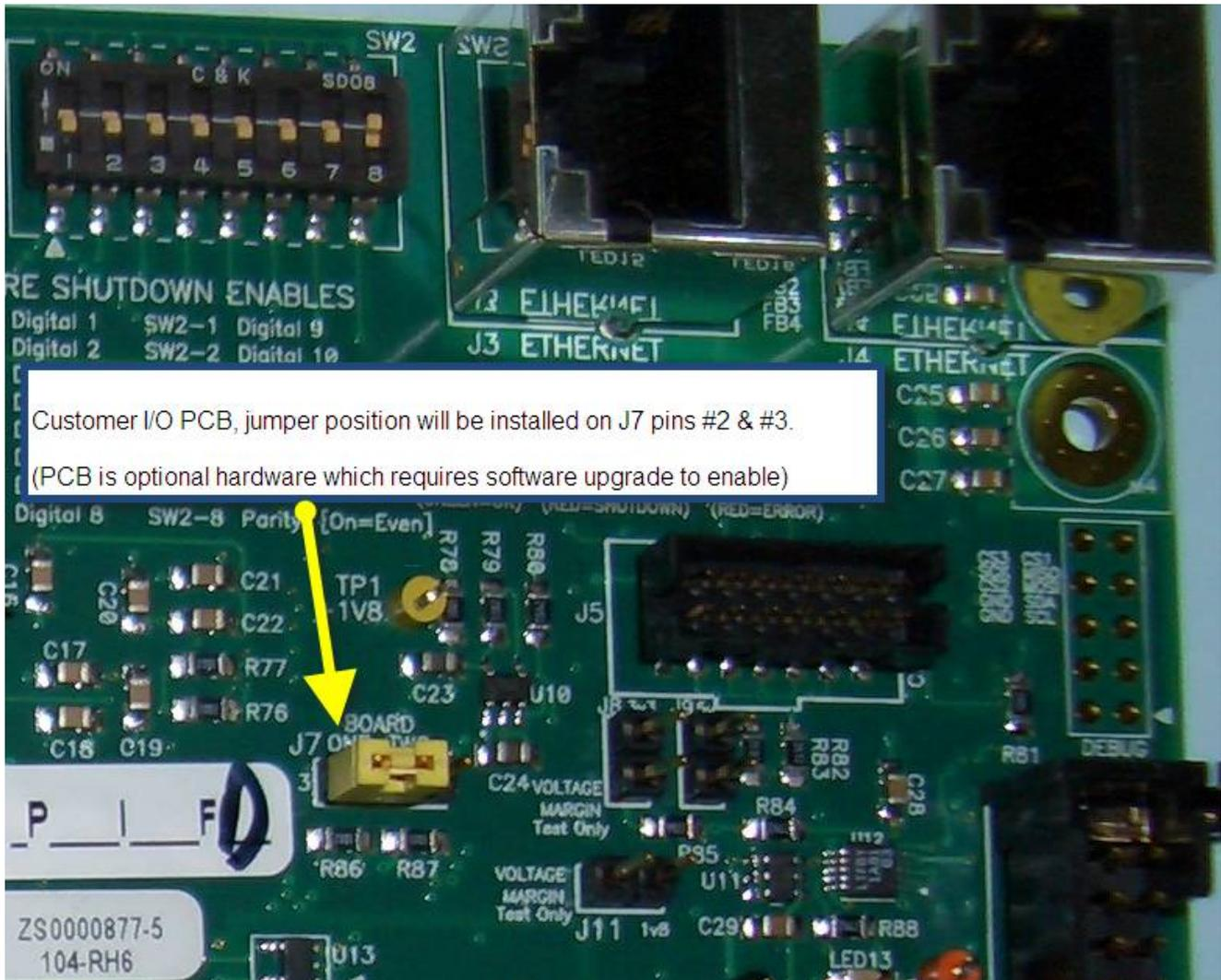
**Figure 2-9:** GASGUARD® AP11 Customer board "J7" jumper configuration.
