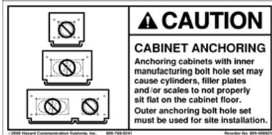
*This symbol cautions against the improper anchoring of cabinets.*
