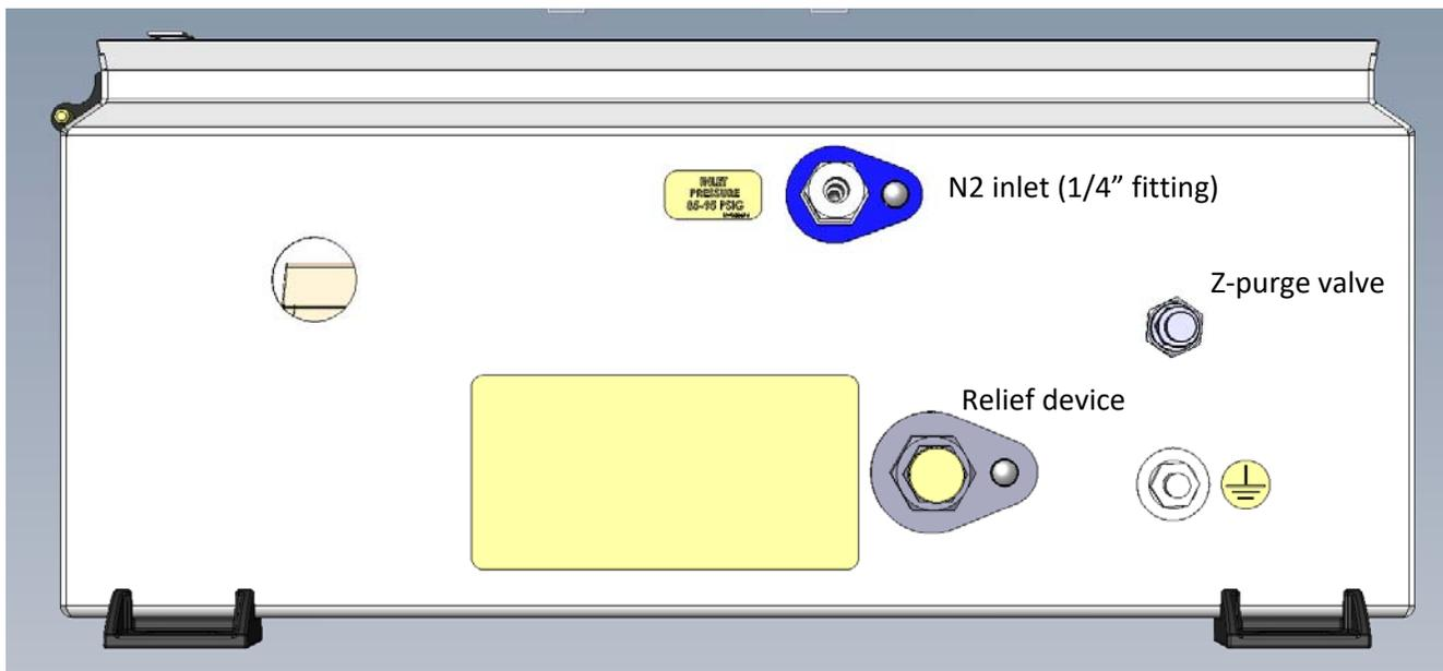
Figure 2-13: Underside View of BSH eV ECC
