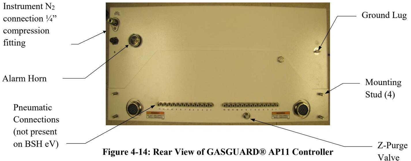
**Figure 4-14: Rear View of GASGUARD® AP11 Controller**
