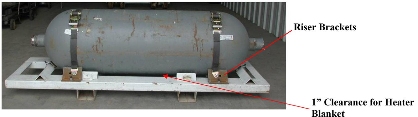
**Figure 4-1: Heating Blanket Configuration.**
