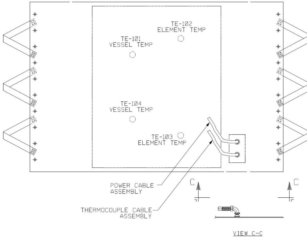
Figure 3-1: Basic layout of Versum Materials Gen II heater blanket
