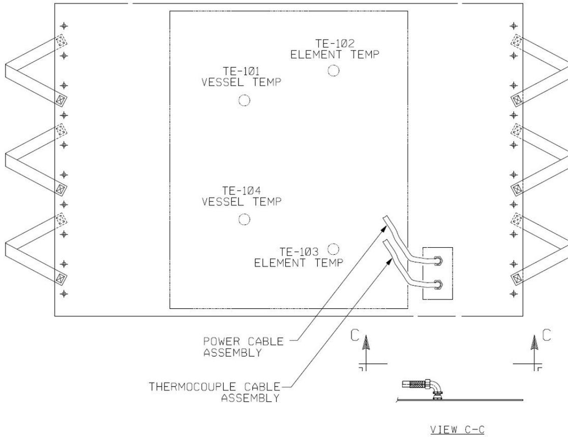
**Figure 4-2: Electric Heater Blanket and Components.**
