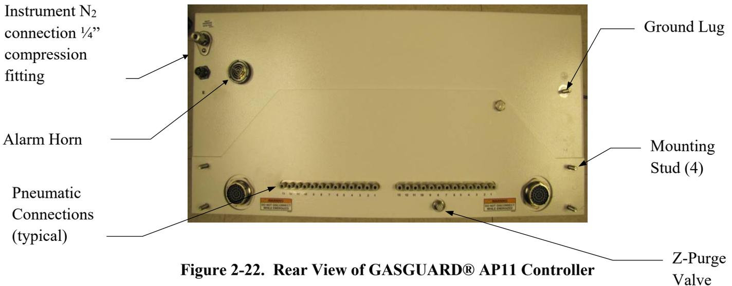
**Figure 2-22. Rear View of GASGUARD® AP11 Controller**
