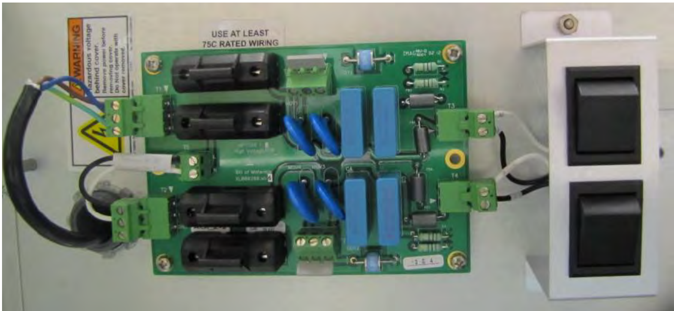
Figure 4.2b: Dual Power Supply Terminal Connection
