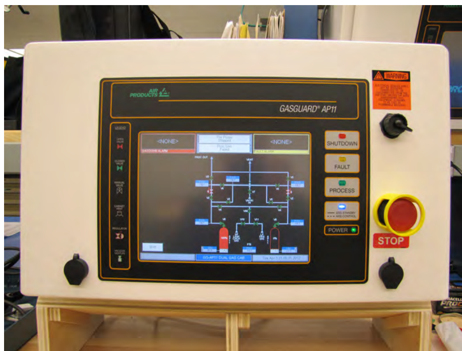
Figure 7.4: GASGUARD® AP11 Controller
