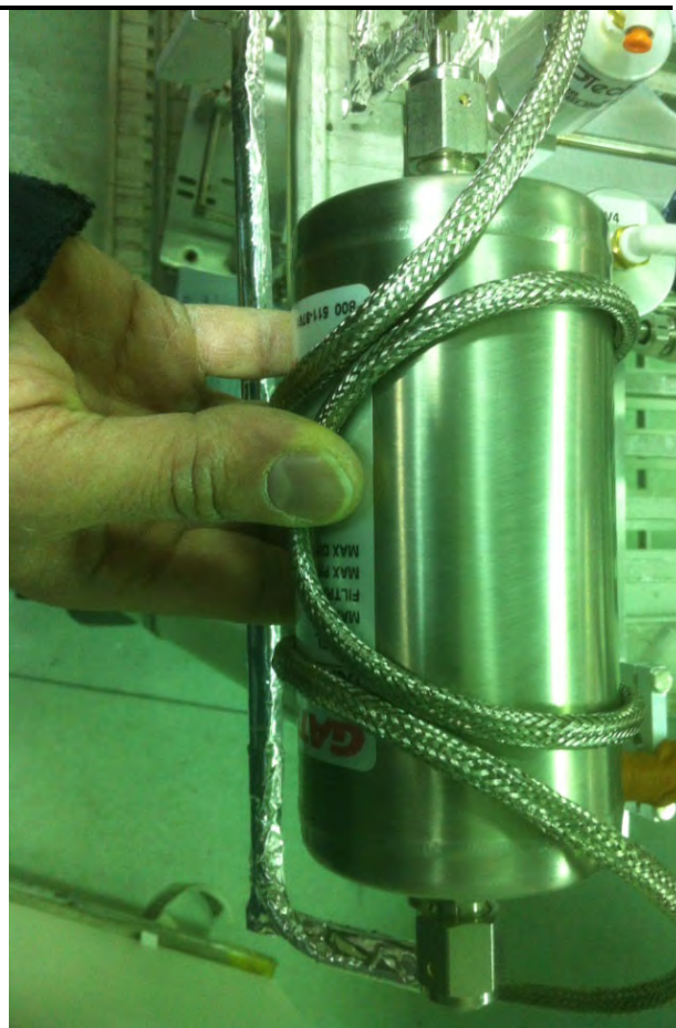
Figure 4: Purifier with cable wrapped around it, before loops are separated and secured.
