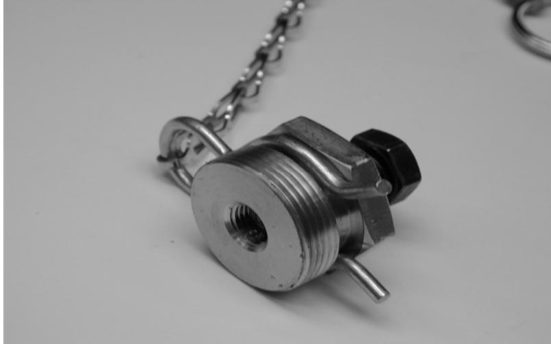
12. Hand-tighten the reset tool into the boost valve. Use an adjustable wrench to hold the boost valve while turning the screw clockwise with a box wrench until it contacts the valve. Continue to turn the screw until a **CLICK/SNAP** is heard. **Do not over-tighten the screw or damage may occur to the boost valve.**
