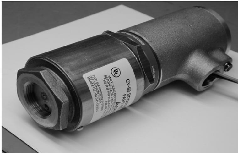
11. Obtain the boost valve reset tool. Before threading the tool into boost valve, back the screw out until approximately .250" TO .375".
