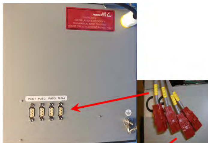
Figure 3-11: PLIS 1-4 DB9 Connectors
