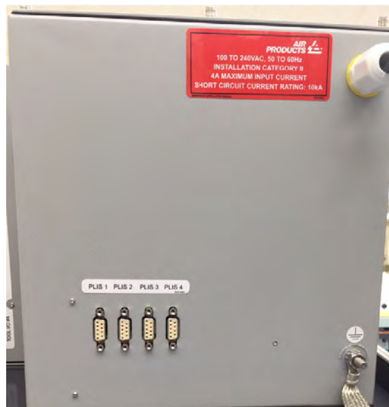
Figure 3-1: Rear View of Conduit Power Entrance
