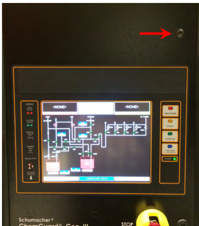
Figure 5-7: Sniffer Port Location
