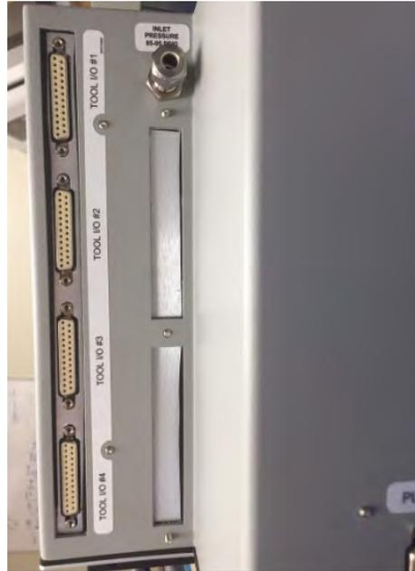
Figure 3-9: Tool I/O Board (AP1614)
