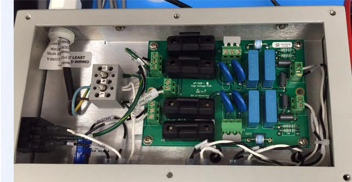
Replaceable fuses - F1, F2, F3, and F4 located on the power board are 4A super quick acting fuses. Also, when a degasser pump is present, a Schurter (p/n # 7022.0700) 10A/500VAC Super Quick Action fuse is located on the inside of the controller.
