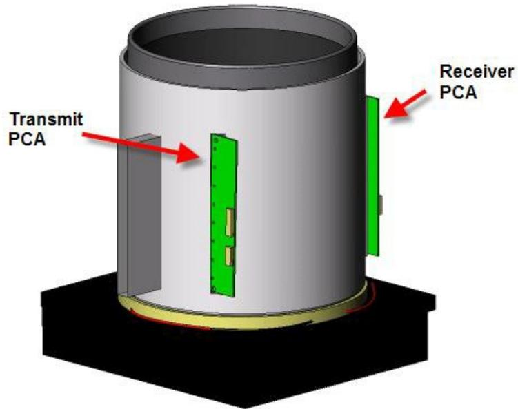
Figure 5-4B Level Detect Positions
