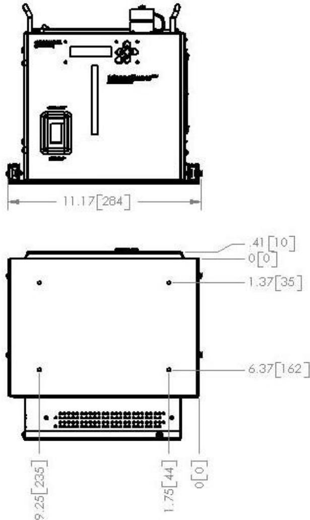
Once installed, the user may pull the Source Cup Assembly by the handles on the top of the Source Cup Assembly. The PEM®'s are for 6-32 screws. The top shelf (not shown) has the same mounting pattern as figure 6.1 above. The screw should not penetrate more than ¼" (0.634 cm) into the assembly.
