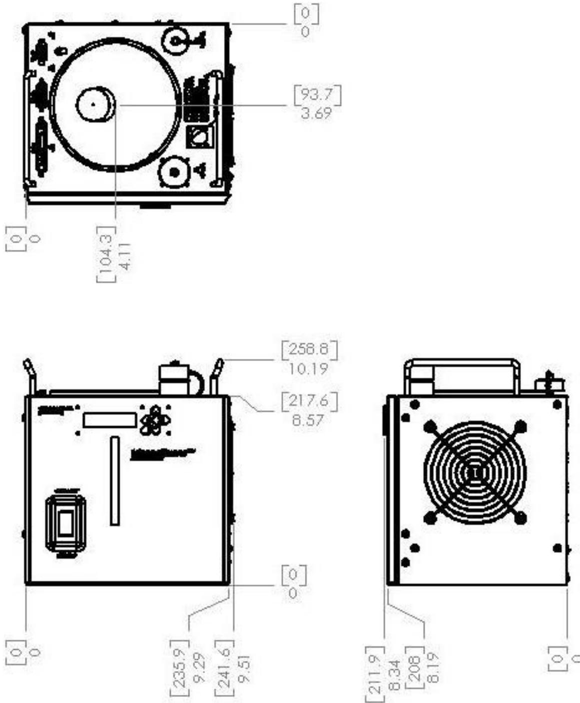
Figure 6-7 Source Cup Assembly, narrow version, inches [mm]
