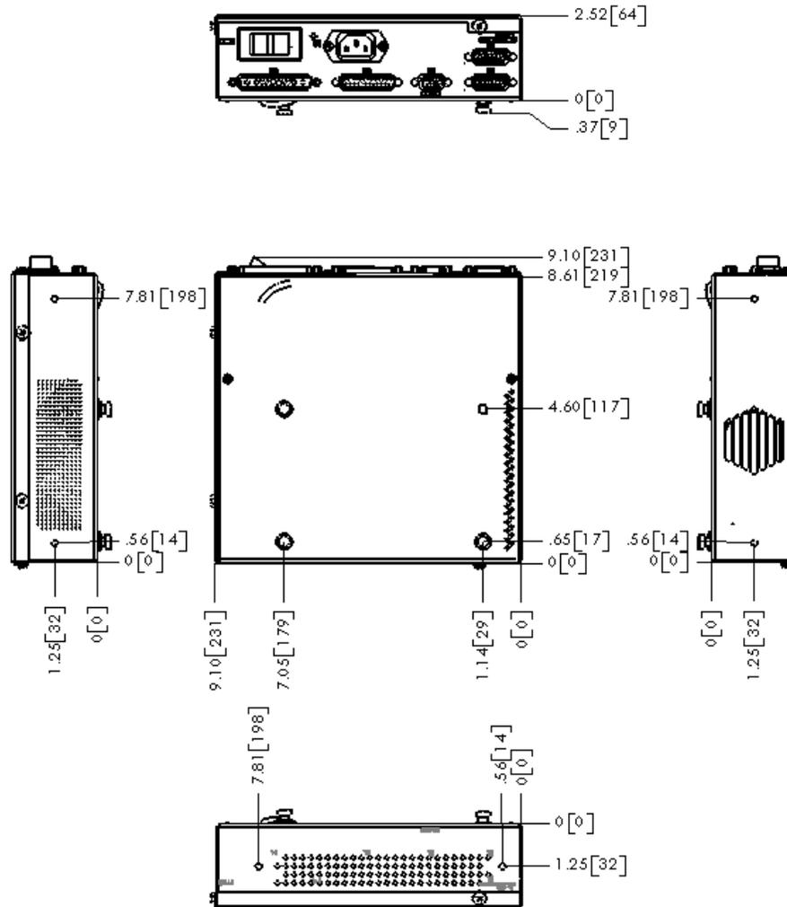
The above figures 6-1 and 6-2 provide the dimensions for seismic mounting for both the Power Supply Module and the Source Cup Assembly. The recommended installation side is the view on the right in figure 6-2 above. Mounting holes were added to two other sides (short sides) to allow for varying installation requirements, however the surface is not flush due to the lid.
