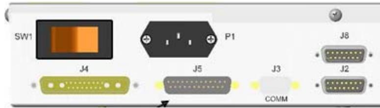
Figure 4.12 Power Supply Module, J5 DDC Cable Connector
