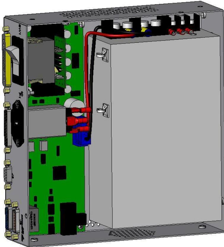
**Figure 5-7a Model 600 Power Supply Module Back Panel**
