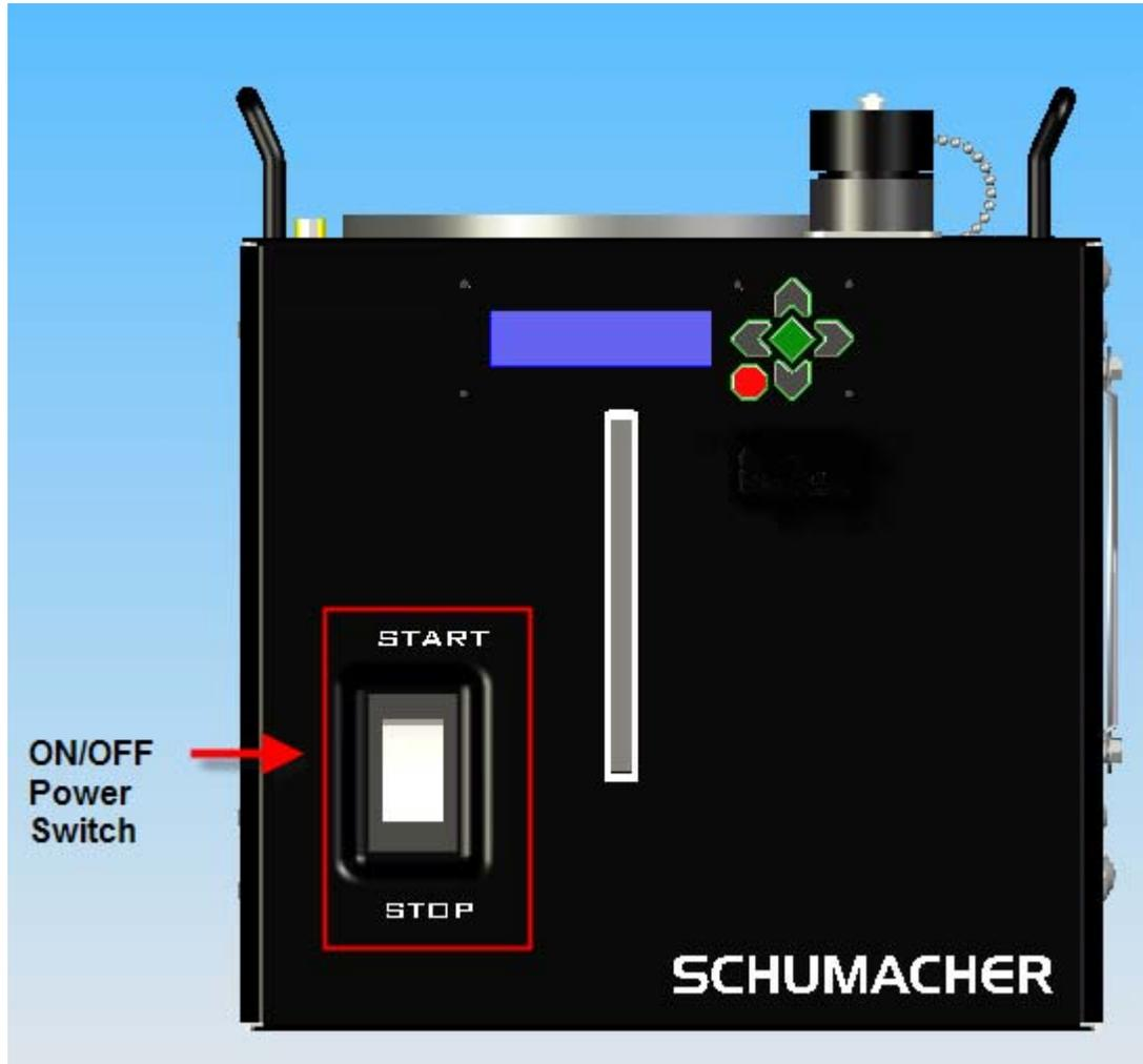
The STOP position of the switch is a hardwired interlock input which the processor monitors. When an alarm condition occurs, the red light will flash. Only an alarm condition will trigger the flashing red LED. When the alarm is cleared, the red light will turn solid red.
