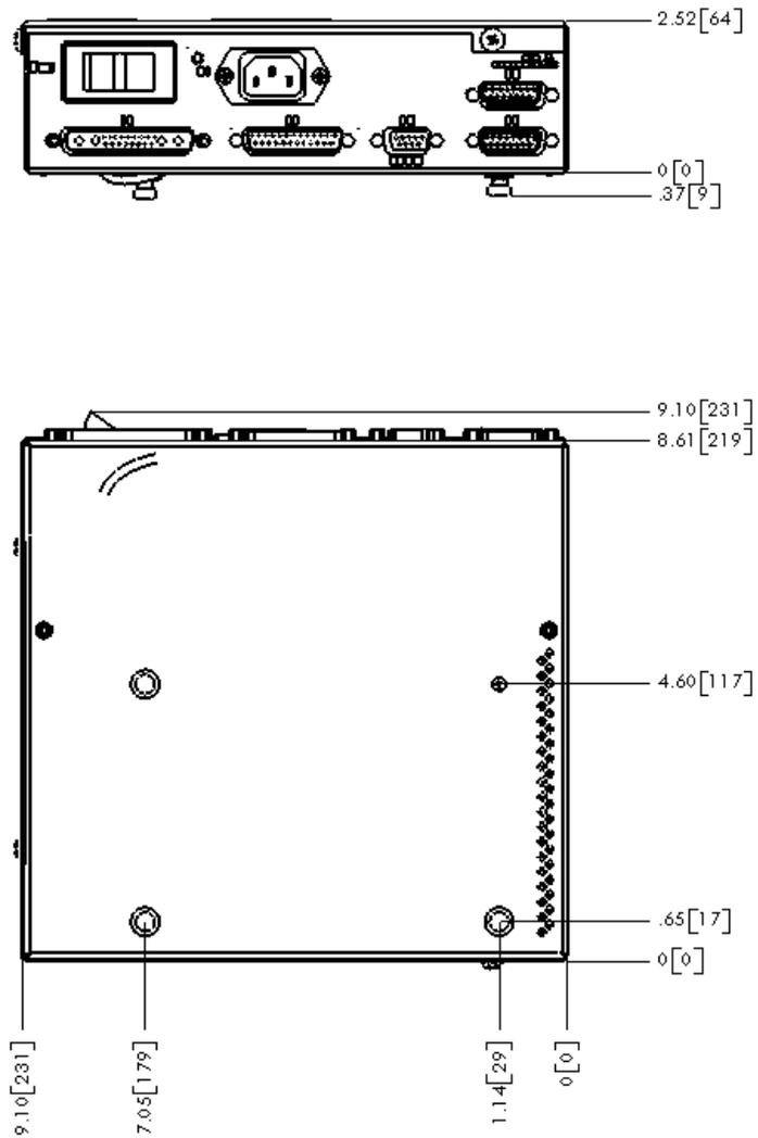
Figure 6-9 Power Supply Module, 300watt, inches [mm]
