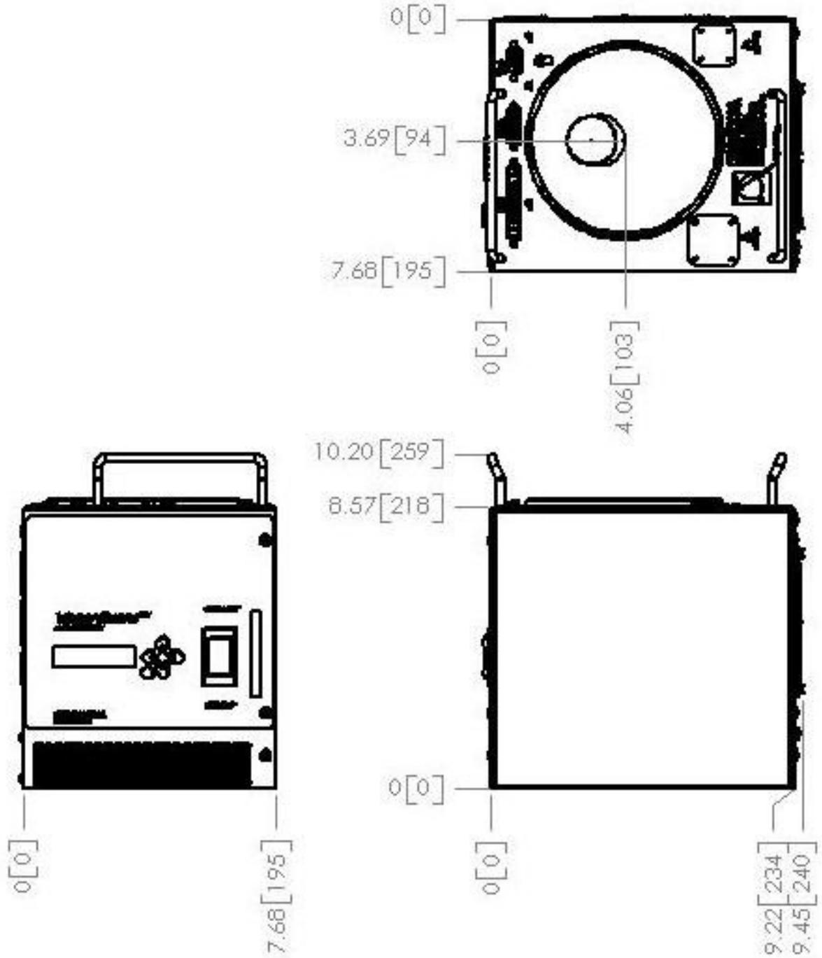
Figure 6-8 Power Supply Module, inches [mm]
