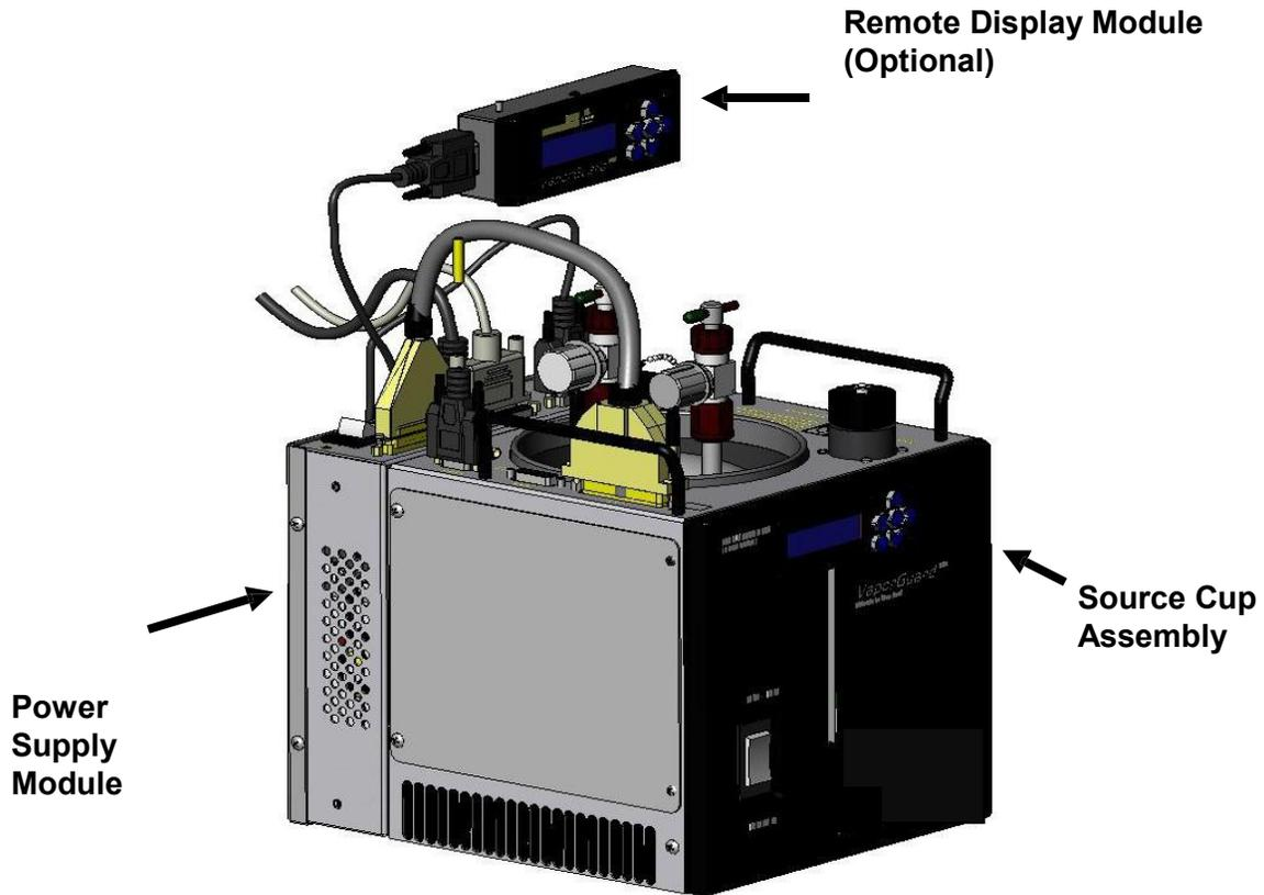
Although the Power Supply Module and Source Cup Assembly processors have separate tasks, they work together to act as one system and communicate between themselves via an RS485 link. The system architecture is implemented in a peer-to-peer configuration.
