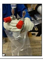
Step 2: Ensure all container valves are closed. Ensure all endcap VCR fittings are closed per Site Form: Closure instructions for Container Valves and Fittings (20422066). Place container into plastic bag zip tie close.
