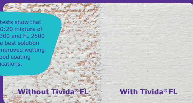
Contaminated wood panel: Right side is perfectly coated with Tivida® FL, while left side without Tivida® FL shows imperfect wetting.
