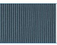
Block Copolymer can generate small lines or contact holes by self-assembly. This allows miniaturization without expensive new equipment.
