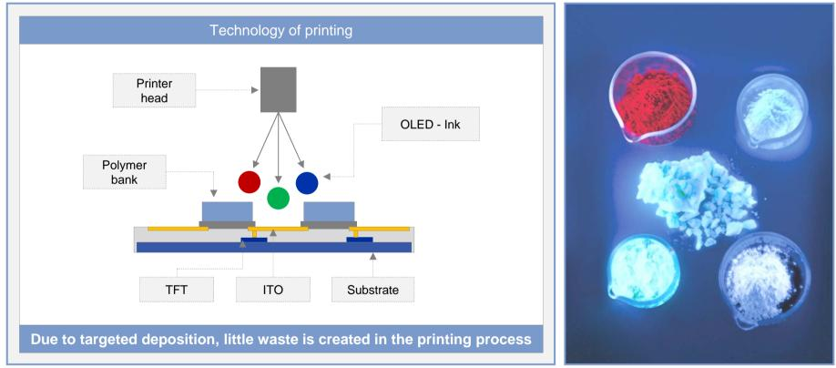
Acronyms: TFT = Thin-film transistor; ITO = Indium tin oxide
