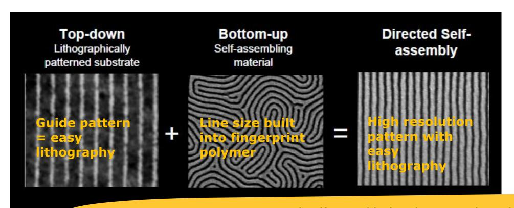
Directed Self-Assembly (DSA) is a paradigm shift in chip making: Only part of the information encoded in a chip layer comes from photolithography, the majority is already embedded in the DSA chemicals.
